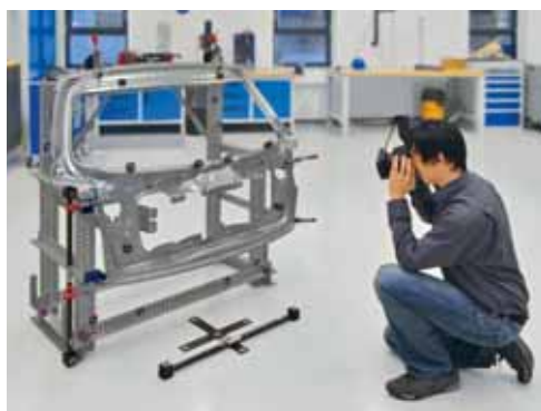
Special coded adapters support the signalisation of boreholes, edges etc.
